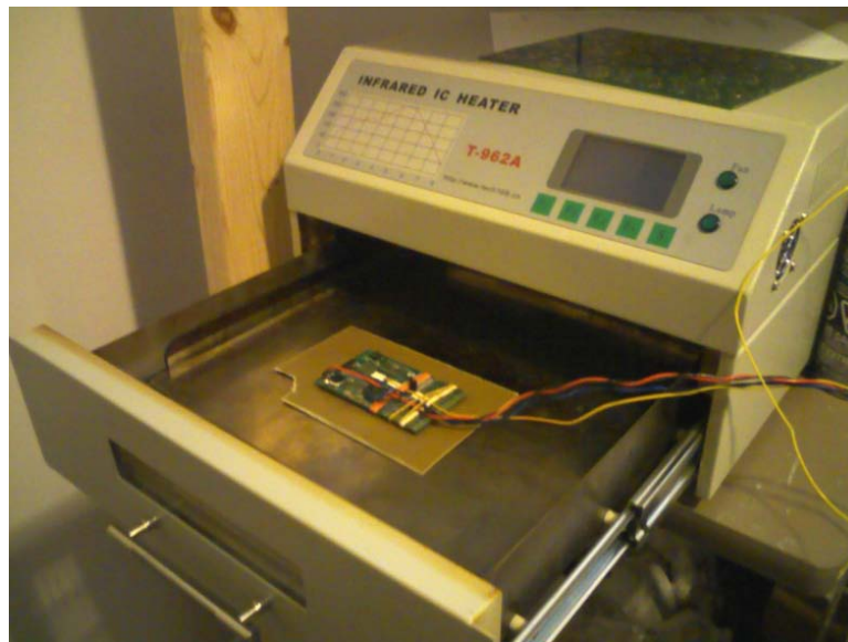
Figure 4: Test Device Inside Infra-Red Oven
